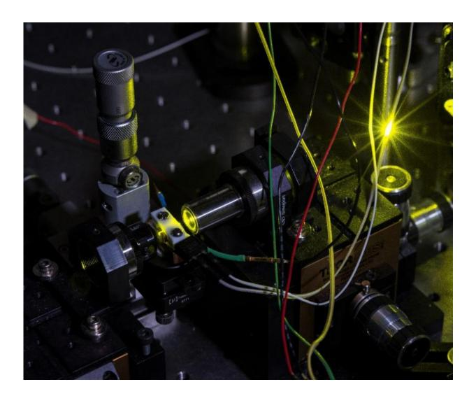
The non-linear crystal, located under the white strip at left of center, up-converts a combination of 1550 nm light and 920 nm light (invisible) to a single output frequency of 577 nm, a bright yellow, while adding almost no noise. Credit: National Institute of Standards and Technology
