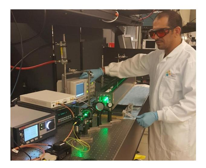
Abdullah Al-Halafi checks the received optical signal power through the underwater channels. Credit: KAUST
