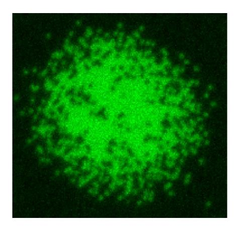
Each green dot represents an individual lithium atom. The researchers use a quantum gas microscope to image the atoms, which have been cooled to a fraction of a degree above absolute zero and trapped in place using lasers. Credit: Peter Brown, Princeton University.
