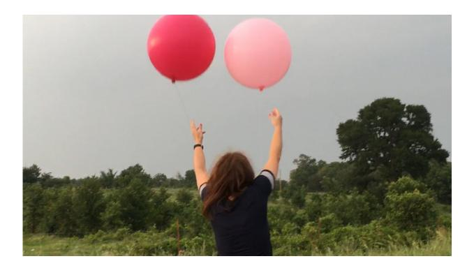
Yvette Richardson, professor of meteorology and associate dean for undergraduate education, Penn State College of Earth and Mineral Sciences launches meteorology probe into storm. The probe is supported by two helium filled balloons that lift it into the air until one balloon is separated from the package so the probe can drift in the storm sending back temperature and humidity data. Credit: Penn State
