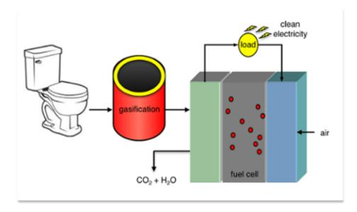
Waste toilet paper can be converted to electricity by gasification followed by reaction with air in a high-temperature fuel cell. Credit: UvA/HIMS
