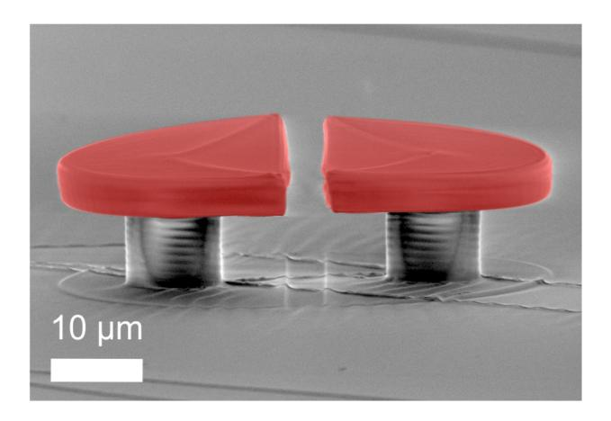
Scanning electron micrograph of a polymeric WGM split-disk cavity: Two opposing half-disks (R=25µm) with an intermediate air gap of several microns are structured onto an elastomeric PDMS substrate with direct laser writing. Credit: Tobias Siegle, Karlsruhe Institute of Technology
