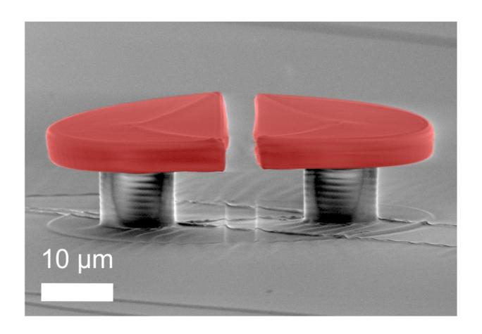
Scanning electron micrograph of a polymeric WGM split-disk cavity: Two opposing half-disks ( $R=25\mu m$ ) with an intermediate air gap of several microns are structured onto an elastomeric PDMS substrate with direct laser writing. Credit: Tobias Siegle, Karlsruhe Institute of Technology
