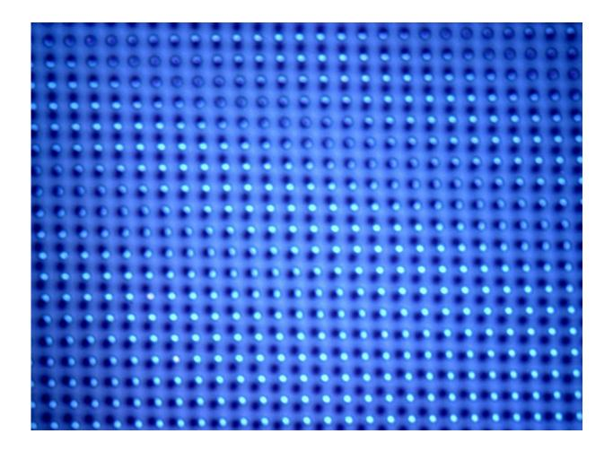
The photograph shows one of the patterned sub-structures that Zhang and his colleagues used in the design of their anti-icing coating. The substructures helped cause macro-cracking at the interface between ice on the surface and the surface itself, a process the researchers called MACI, for macro-crack initiator. Credit: NTNU Nanomechanical Lab
