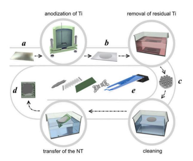
The scheme of fabrication the multisensor chip based on TiOx NT array: (a–e) denote respectively Ti foil (a), Ti foil with as-prepared NT array (b), the extracted NT array (c), the NT array placed over the chip (d), the scheme of multisensor chip wired into 50-pin ceramic card (e) Credit: *Scientific Reports*
