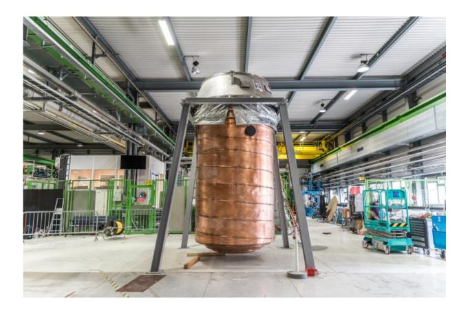
The FRESCA2 cryostat before the insertion of the magnet. Credit: Sophia Bennett
