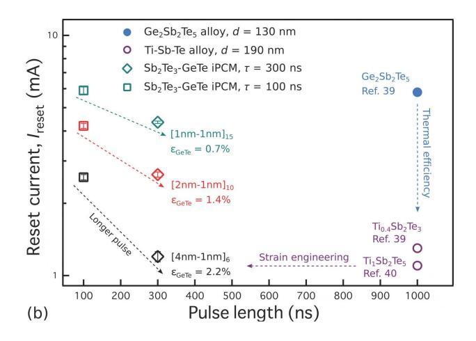
A comparison of the electrical switching current and switching times for the strained superlattices interfacial phase change memory with other state-of-the-art phase change memory materials. Credit: Zhou et al.
