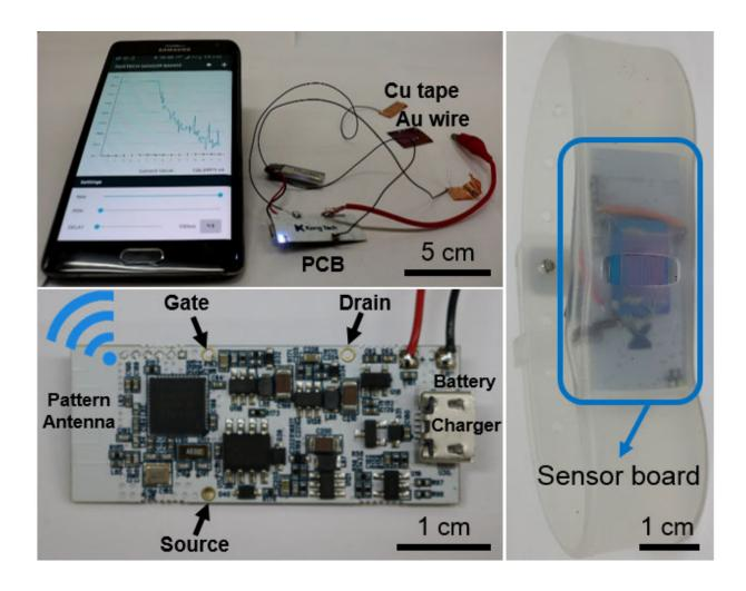
This figure represents the newly developed amphetamine sensor with a wireless communication system. The drug sensor consists of a highly sensitive organic transistor platform functionalized with drug-specific host molecules. Credit: Jang et al.
