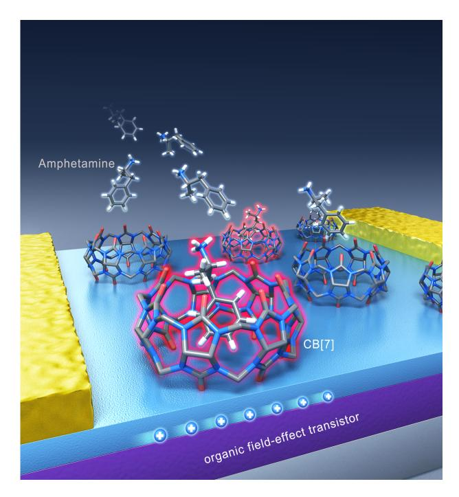
Binding of drug molecules to the hollow cucurbit[7]uril (CB[7])'s cavity changes the current signal flowing in the transistor and therefore can be used as a detection system. The molecular structure of amphetamine and methamphetamine bound to cucurbit[7]uril (CB[7]) was confirmed with X-ray crystallography. Each color indicates a different atom (blue: nitrogen, red: oxygen, gray: carbon, and white: hydrogen). CB[7]'s hydrogen atoms have been
