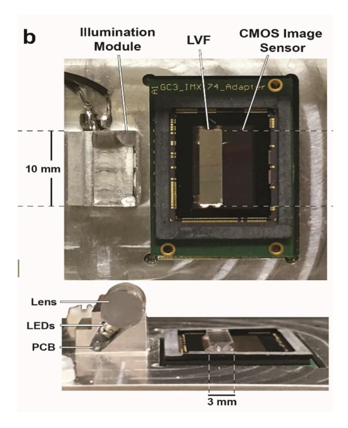
Top view and side view of the compact spectrometer for the smartphone science camera, comprised of an image sensor chip with a linear variable filter attached
