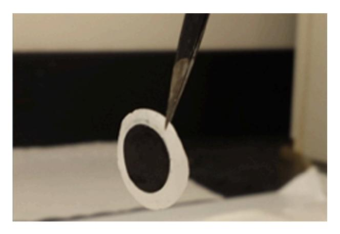
This carbon nanofiber electrode, when coated with ionogel, can eliminate the need for a flammable electrolyte solution in energy storage devices -- making them safer to use. Credit: Drexel University
