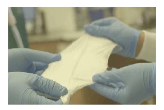
Drexel researchers have developed a solid-state, free-standing electrode that can make energy storage devices safer by eliminating their flammable electrolyte solution. The electrode uses a carbon fiber mat, made by the process of electrospinning shown here. Credit: Drexel University
