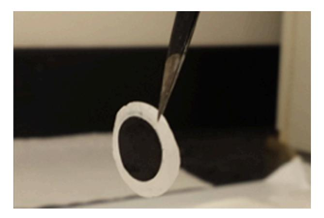
This carbon nanofiber electrode, when coated with ionogel, can eliminate the need for a flammable electrolyte solution in energy storage devices -- making them safer to use. Credit: Drexel University
