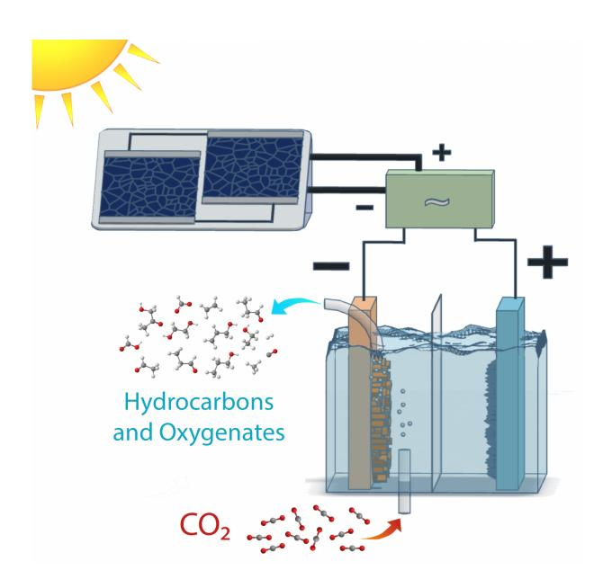
Schematic of a solar-powered electrolysis cell which converts carbon dioxide
