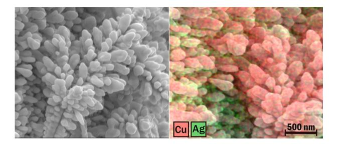
At left is a surface view of a bimetallic copper-silver nanocoral cathode taken from a scanning electron micrograph. To the right is an energy-dispersive X-ray image of the cathode with the copper (in pink/red) and silver (in green) highlighted. Credit: Gurudayal/Berkeley Lab
