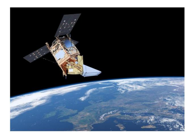
Sentinel-5 Precursor is the forerunner of Sentinel-5 to provide timely data on a multitude of trace gases and aerosols affecting air quality and climate. These data will be used for air-quality monitoring services through Europe's Copernicus programme. Sentinel-5 Precursor carries an imaging spectrometer called Tropomi. Credit: ESA/ATG medialab
