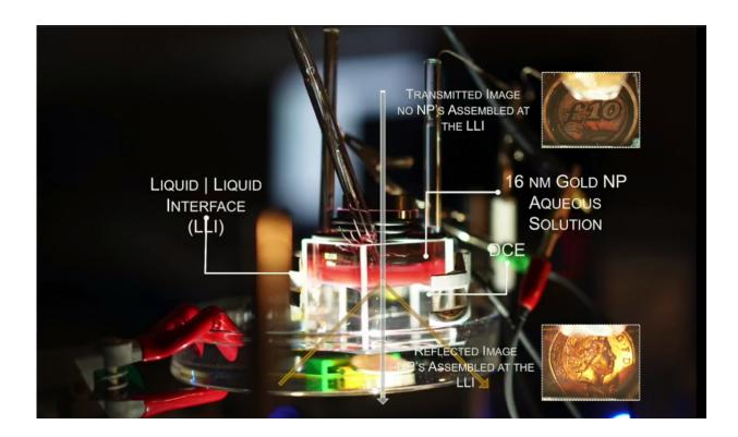
By finely tuning the distance between nanoparticles in a single layer, researchers have made a filter that can change between a mirror and a window.
