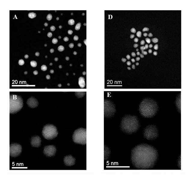
Representative HAADF images and particle size distributions for the unsupported AuPd-PVP sol in the fresh (A to C) and after a CH4 oxidation
