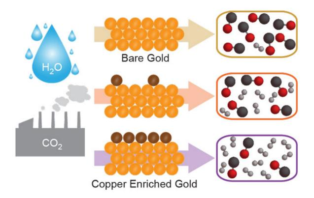
Schematic depicting the production of syngas from carbon dioxide and water. Bare gold catalysts make syngas mixtures that are rich in carbon monoxide, whereas gold catalysts enriched with copper make syngas mixtures that are more hydrogen rich. Credit: Michael Ross/Berkeley Lab
