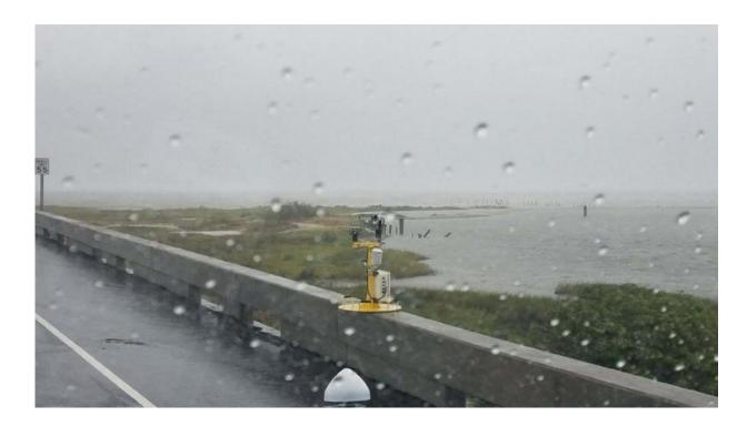
A weather pod deployed on a bridge north of the Doppler on Wheels. It tracked Harvey's winds. Credit: Center for Severe Weather Research
