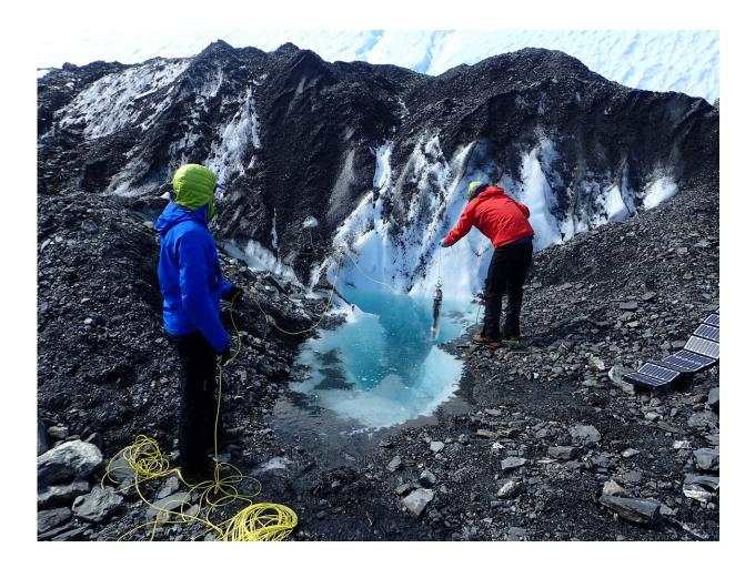
JPL engineers Andy Klesh and John Leichty lower a homemade probe into a moulin on Alaska's Matanuska Glacier. Along with a robot submersible, this probe helped them build 3-D maps of the underwater tunnel systems within the glacier. Credit: NASA/JPL-Caltech
