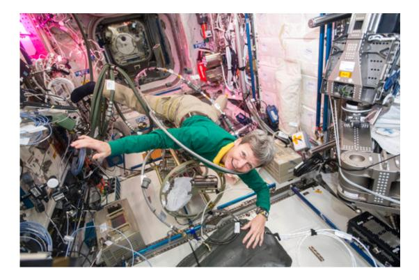
In this Dec. 8, 2016 photo made available by NASA, astronaut Peggy Whitson floats through a tangle of cables inside the Columbus module aboard the International Space Station. Whitson was operating the Fluids System Servicer to refill coolant loops in multiple modules on the U.S. segment of the station. (NASA via AP)
