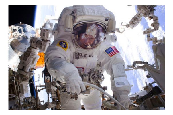
In this Jan. 6, 2017 made available by NASA, astronaut Peggy Whitson works during a spacewalk outside the International Space Station. Whitson and fellow astronaut Shane Kimbrough successfully installed three new adapter plates and hooked up electrical connections for three of the six new lithium-ion batteries on the ISS. (NASA via AP)
