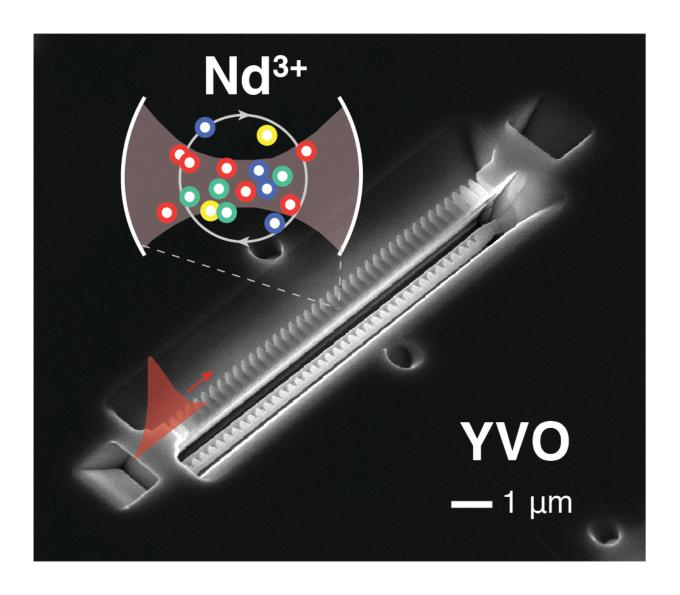
Scanning electron microscope image showing the nano-scale optical quantum memory fabricated in yttrium orthovanadate (YVO). The schematic shows that this device is an optical cavity that contains Nd atoms. Credit: Dr. Tian Zhong
