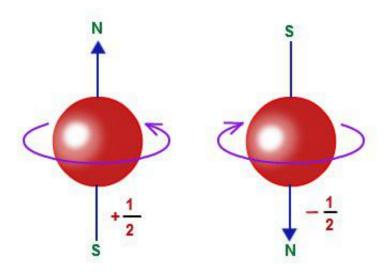
Fig. 1. The term "spin" refers to the intrinsic angular momentum of a particle. The spin of a particle has both a magnitude and a direction. In the case of the electron, the magnitude is 1/2 times Planck's constant, and the direction is either up or down. Credit: 10.1103/PhysRevLett.119.107601
