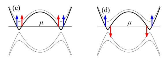
Fig.2. In the figure, electron and hole energy is plotted against momentum. (The four black curves correspond to two projections of electron spin and two projections of hole spin.) The thick curve corresponds to electron states capable of conducting an electric current (forming a Fermi surface). Depending on the mutual orientation of the spins of electrons (blue arrows) and holes (red arrows) on the Fermi surface, the system is either an ordinary half-metal (c) or a spin-
