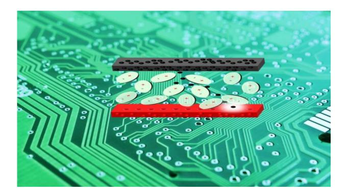
Blending polymer materials in the right combination can create fractional-order capacitors that are compatible with printed circuit boards. Credit: KAUST
