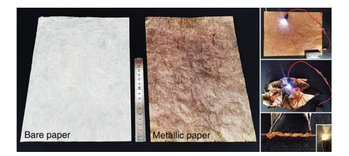
Photographs of the original paper and the paper coated with gold nanoparticles, which can be used to light LEDs. Credit: Ko et al. Published in *Nature Communications*.
