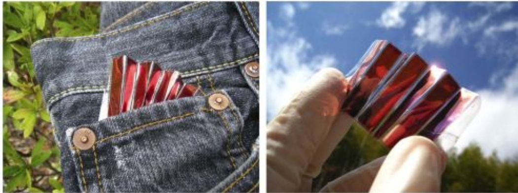
Figure 1: Portable paper solar cells based on foldable, lightweight, transparent, conductive cellulose nanofiber paper. Credit: CC-BY Macmillan Publishers Ltd
