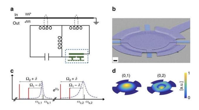
Implementation of a superconducting microwave circuit optomechanical device for nonreciprocity. Credit: *Nature Communications* (2017). DOI: 10.1038/s41467-017-00447-1
