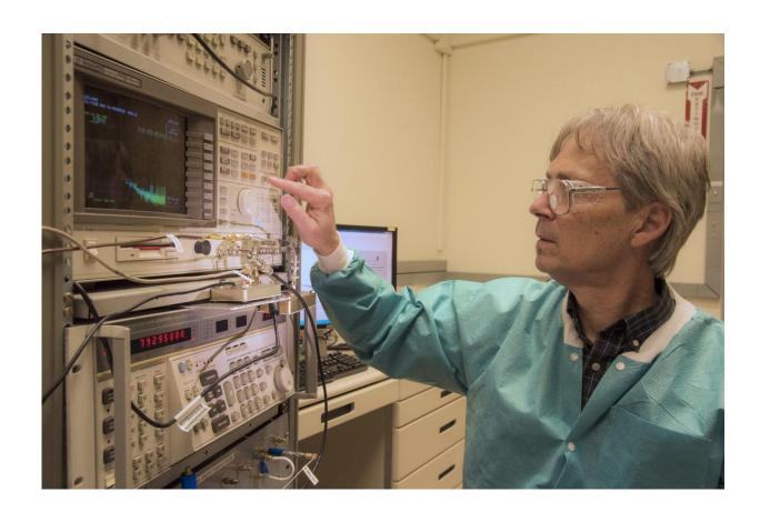
NIST physicist Ward Johnson observes signals generated by bacteria coating quartz crystals, a novel method of sensing whether an antibiotic kills the bacteria. The new NIST technique senses mechanical fluctuations of bacterial cells and any changes induced by an antibiotic. With further development, the technique could hasten the identification of effective medical treatments in clinical settings and drug development. Credit: Burrus/NIST
