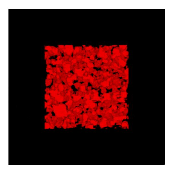
3-D rendering of the nanoparticle bijel taken by confocal microscope. Credit: Caili Huang/ORNL and Joe Forth/Berkeley Lab
