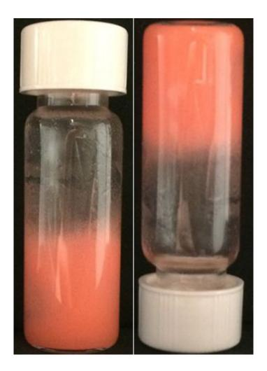
At left is a vial of bijel stabilized with nanoparticle surfactants. On the right is the same vial after a week of inversion, showing that the nanoparticle kept the liquids from moving. Credit: Caili Huang/ORNL
