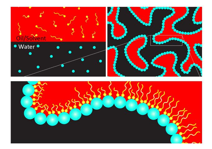
This illustration shows key stages of bijel formation. Clockwise from top left, two non-mixing liquids are shown. Ligands (shown in yellow) with amine groups are dispersed throughout the oil or solvent, and nanoparticles coated with carboxylic acids (shown as blue dots) are scattered in the water. With vigorous shaking, the nanoparticles and ligands form a 'supersoap' that gets trapped at the interface of the two liquids. The bottom panel is a magnified view of the
