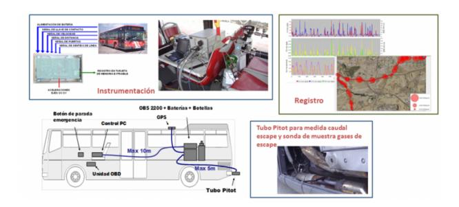
On-board instrumentation equipment on a bus and collection and data recording. Credit: INSIA
