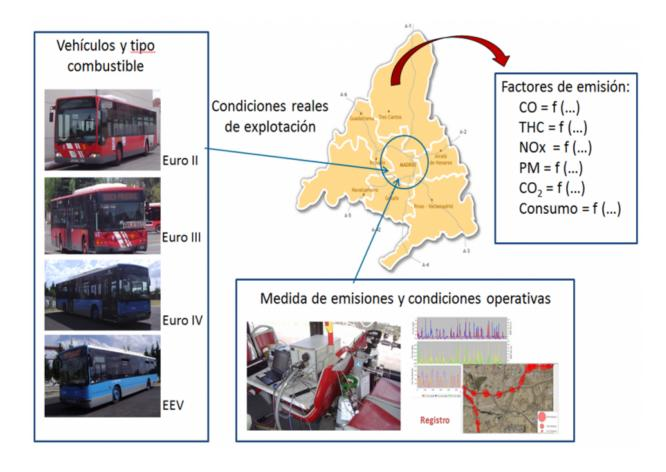
Methodology applied to obtain the model of emissions and fuel consumption of urban bus fleets. Credit: INSIA
