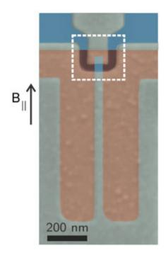
One of the nanowires central to the NBI-scientist's research. The wire is made out of aluminum. It is approx. 1/1.000 millimeter long, and 1/20.000 wide. Credit: NBI
