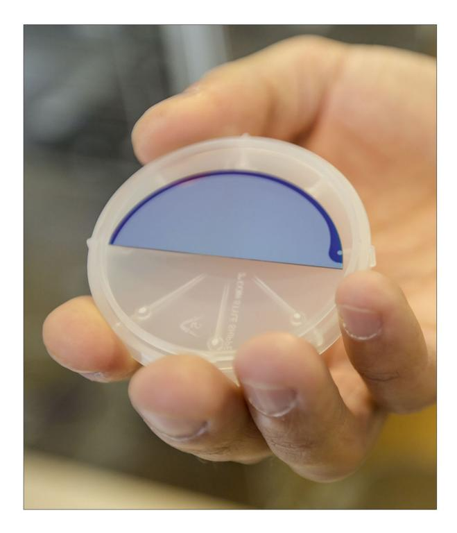
The blue part of the structure—one half of a wafer—is where the scientists start building the nano wire. Credit: Ola Jakup Joensen
