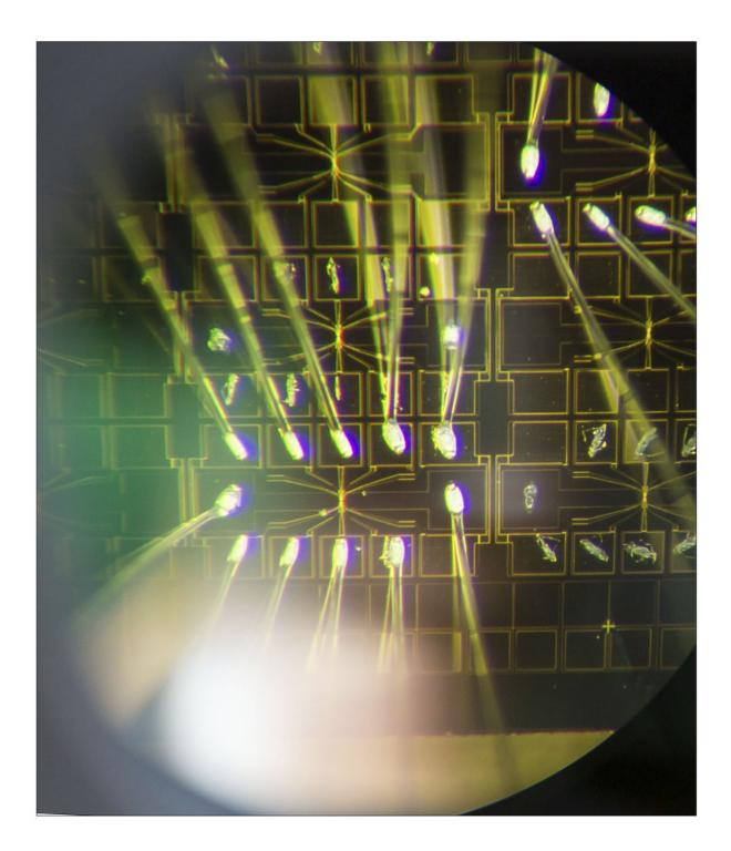
The nano wire is embedded in spider shaped structures. These structures are here seen through the lense of an optical microscope. The structures sit in rows, two in each row. Credit: Ola Jakup Joensen
