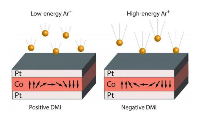
Schematic shows how different energies of argon (Ar) ions bombarding a thin film of cobalt (Co) sandwiched between platinum (Pt) layers can twist or rotate the spin of electrons in a particular direction, by controlling an effect known as the Dzyaloshinskii-Moriya interaction (DMI). Credit: NIST
