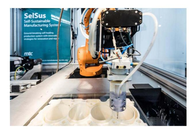
Self-repairing dispenser for engine production developed within the EU-funded SelSus research project by project partner Manufacturing Technology. Credit: Fraunhofer IPA
