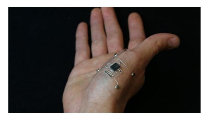
A complete hybrid 3D-printed device flexes and conforms to the body's shape. Credit: courtesy of the Wyss Institute for Biologically Inspired Engineering
