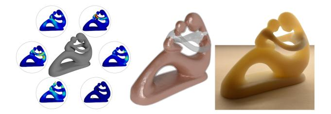
Critical instant analysis, a new process for improved structural optimization in additive manufacturing, unveils the possibility of designing products that are lighter in weight and cheaper to produce. Credit: Burak Kara and Erva Ulu, Department of Mechanical Engineering, Carnegie Mellon University
