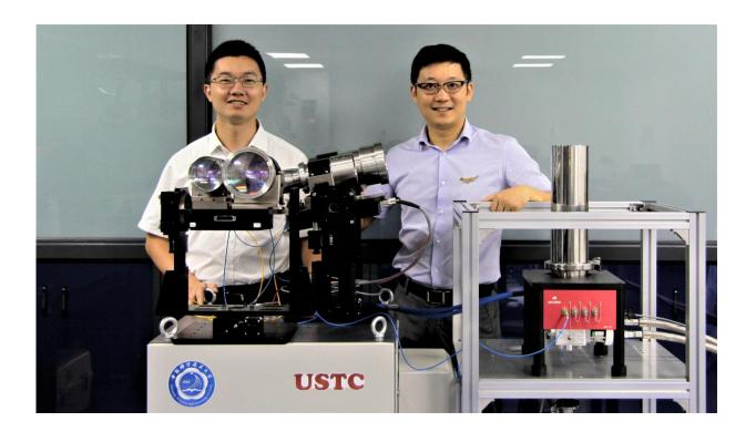
Mingjia Shangguan and Haiyun Xia from the University of Science and Technology of China were part of a research team who developed a new Doppler LIDAR system for accurately measuring the wind. It features a greatly simplified optical setup that makes it robust and stable enough to use in harsh environments such as aboard aircraft or satellites. Credit: Quantum LIDAR Laboratory
