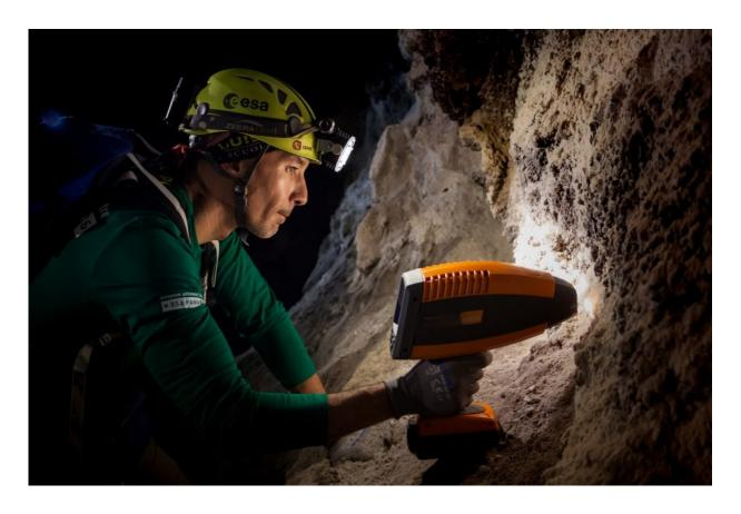
Checking the mineral composition of some weathered rocks with the HaloSpec Spectrometer during ESA astronaut PANGEA training course in terrestrial lava tubes in Lanzarote. Credit: ESA/L. Ricci
