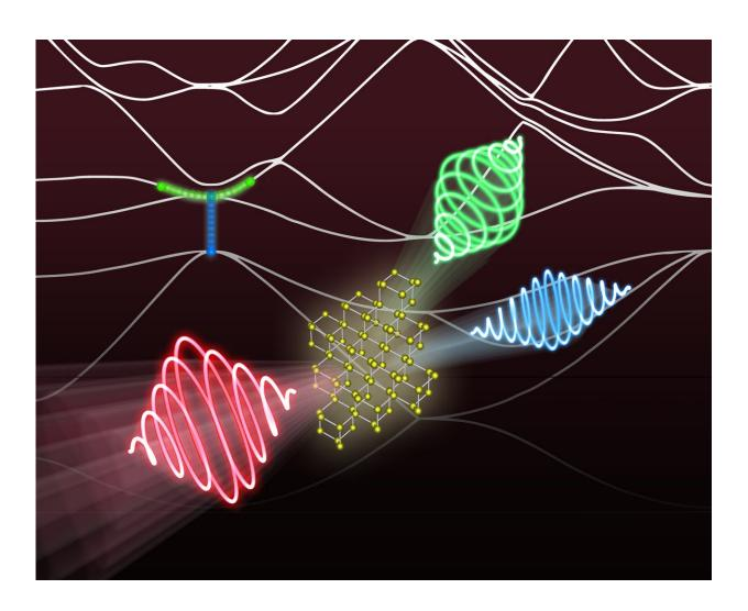
When exciting crystals such as silicon by an intense elliptically or circularly polarized light pulse (red), circularly polarized higher harmonics (green & blue) can be generated. Credit: Nicolas Tancogne-Dejean + Joerg M. Harms, MPSD
