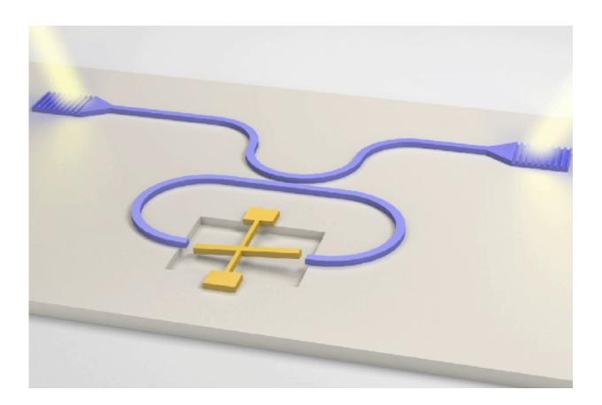
Schematic (animated) of torsional optomechanical resonator for sensing and frequency mixing. Credit: Jianguo Huang
