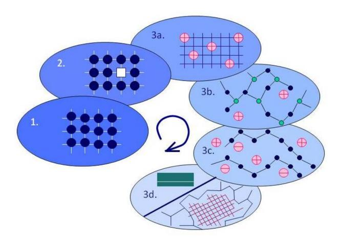
Evolution of materials used in solid-state ionics: 1 – ideal crystals; 2 –crystals with point defects; 3a – crystals with structural disorder; 3b – ion-conducting glasses; 3c – polymer electrolytes; 3d –nanosized systems. Credit: National Institute for Materials Science
