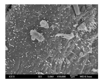
A scanning electron microscope image showing the quercetin nanoparticles bonded to the surface of the cellulose fiber. Credit: A\*STAR Institute of Chemical and Engineering Sciences
