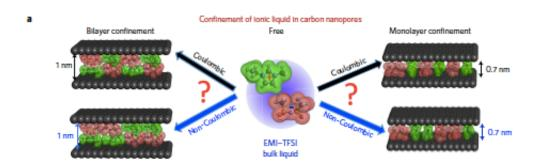
When packed into pore channels as narrow as a nanometer or less, ions will forgo their typical positive-negative alternating charge ordering. They will form a single (right) or double-file (left) line, many times queuing up next to ions of the same charge. Credit: Drexel University
