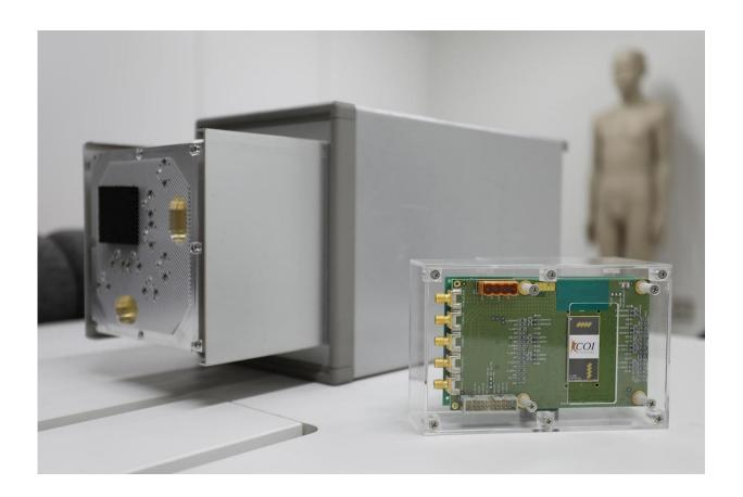
KU and Panasonic developed a radar-based device that could instantaneously and accurately measure the body's vital signals. The new model is smaller and more accurate than its predecessor. Credit: Kyoto University
