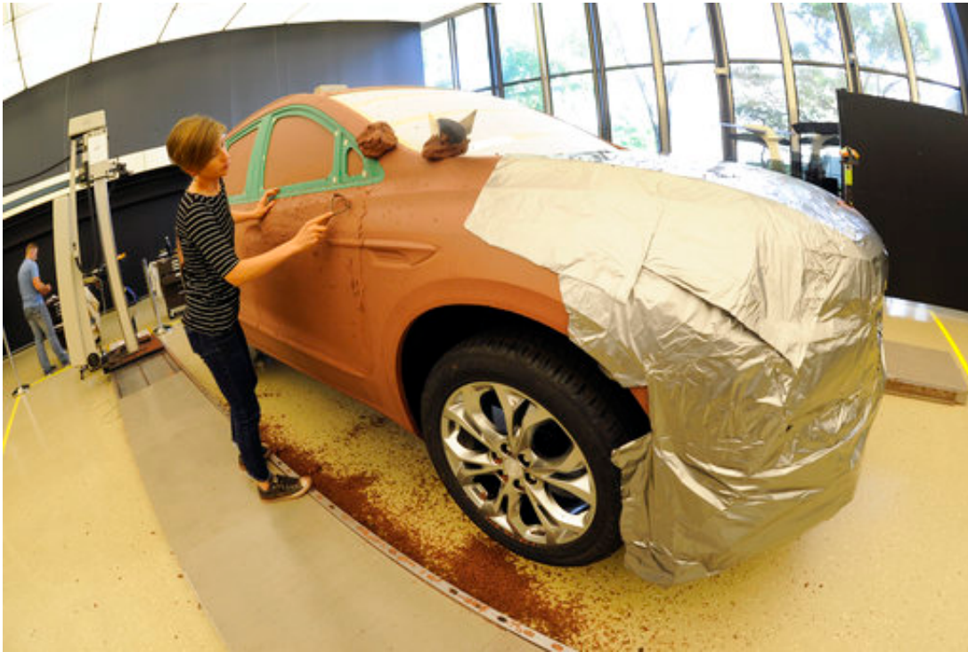
General Motors creative clay sculptor Gianna Ball smooths loose clay on a model of a 2018 Buick Enclave frame, Friday, Aug. 25, 2017 at the GM Tech Center in Warren, Mich. (AP Photo/Jose Juarez)
