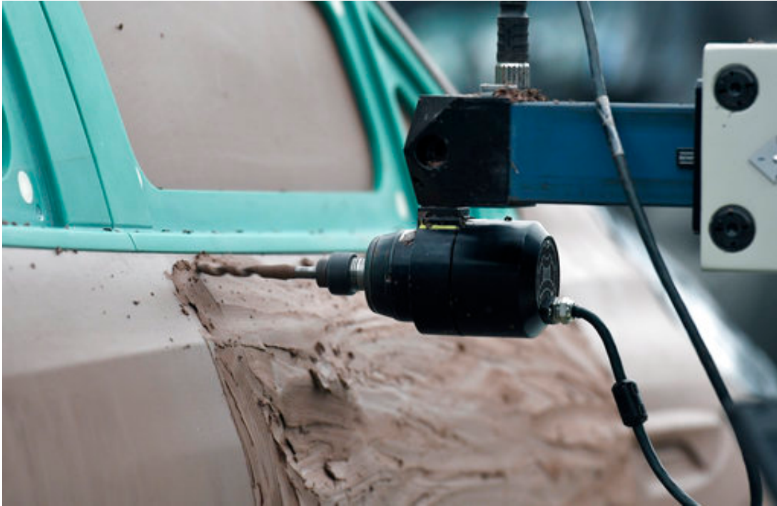
A Tarus three axis machine mills the clay on a passenger door of a 2018 Buick Enclave, Friday, Aug. 25, 2017 at the GM Tech Center in Warren, Mich. (AP Photo/Jose Juarez)
