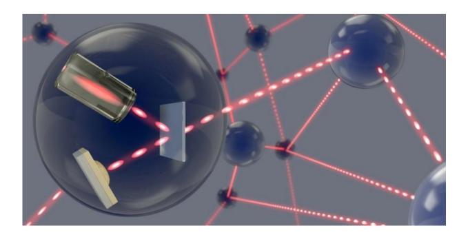
Schematic of a quantum network: single photons transmit quantum information between the network nodes, where they are stored in an atomic gas. Credit: University of Basel, Department of Physics
