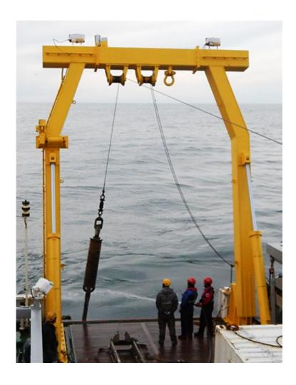
A sediment core has been captured in the steel gravity core barrel that is below the 1,500-kilogram lead weights (pictured to the left of the people) and retrieved at the R/V Araon's stern. Credit: Monterey Bay Aquarium Research Institute
