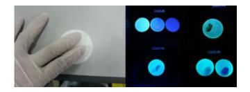
The polymer-coated polymer readily could detect fingerprints contaminated with traces of four common high explosives, including TNT. Credit: The Royal Society of Chemistry
