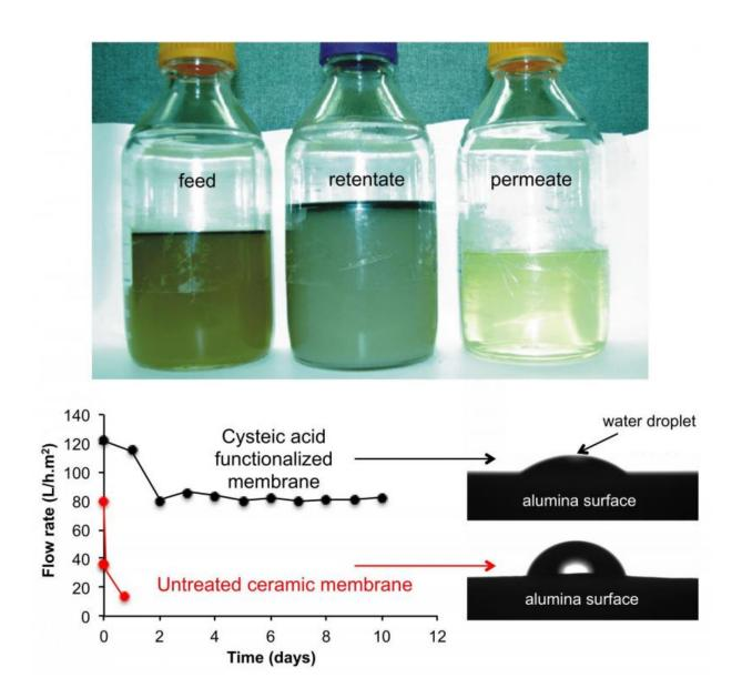
A superhydrophilic filter produced at Rice University can remove more than 90 percent of contaminants from water used in hydraulic fracturing operations. In this image, "produced" water from a Marcellus shale fracturing site is at left, the
