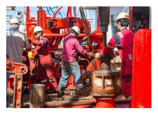
To collect sediment cores from deep beneath the seabed we need a drill that may be more than 5000 metres long and weigh more than 200 tonnes. Credit: Tim Fulton, IODP/TAMU, CC BY-ND
