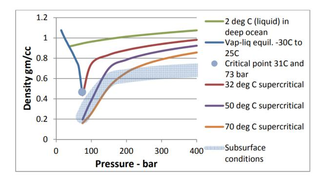
Density vs. pressure for CO2 at subcritical and supercritical conditions. Credit: *Energy Procedia* (2017). DOI: 10.1016/j.egypro.2017.03.1686
